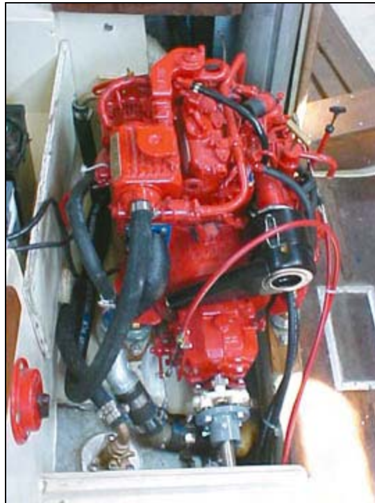
This new Beta 14 diesel engine, installed in a Tartan 30, replaced a tired Atomic 4 gasoline engine.
