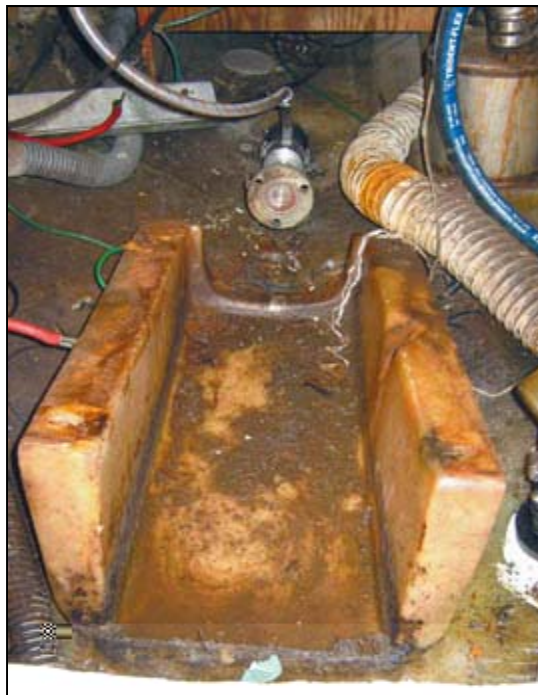
With the old engine removed, it's a good time to clean and paint the engine compartment.
